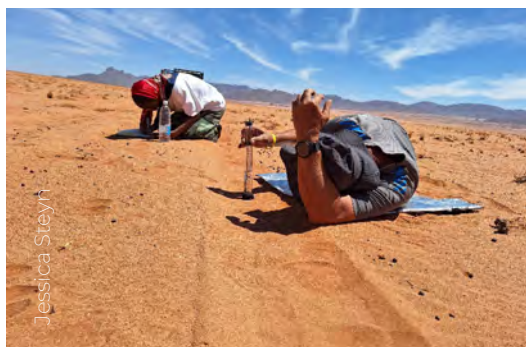
Measuring the water infiltration rate on vehicle tracks
