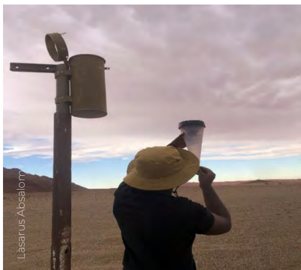
Checking the rain gauges for rainfall
