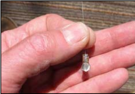
Plate 3: Radio transmitter built especially for us by Blackburn Transmitters (Nacogdoches, Texas 75961). They measured 12 x 5 x 4 mm and weighed 0.3 g. The 7.0 cm-long whip antenna is made of nylon-coated stainless steel fishing leader wire (7x7 Surflon Micro Supreme 20 lb. test). To maximize transmitter life (nearly 30 days), we used a three second pulse interval. © G.B. Rathbun
